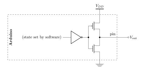
The transistors in the output pin have non-negligible on resistance, so aren't suitable for driving large loads. When talking about this resistance in relation to an output pin, we call it the *output resistance* of the pin—in other words, the resistance "seen" by a device connected to the pin. Since this resistance might depend on the state of the pin (HIGH or LOW), it actually has two output resistances. You'll measure both in prelab 2b.
