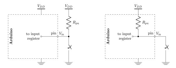
As you might guess, the internal pull-up resistor itself is enabled using a PMOS transistor. Thus, here is a (simplified) schematic of an input pin:
