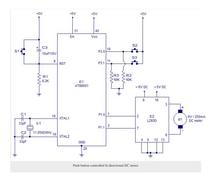
The code for the above project is so written that initially when power is switched ON, the motor remains OFF. When push button switch S2 is pressed P1.0 goes high and P1.1 remains low. The motor runs in the clockwise direction and this condition is maintained until S3 is pressed. When push button switch S3 is pressed the logic of P1.0 and P1.1 toggles making the motor to run in the opposite direction and this condition is maintained until the next press of S2.
